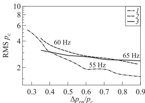
**Figure 8** Double time lag,  $\Delta p_{fu}/p_c = 0.5$ ; chamber pressure RMS vs. oxidizer injector pressure drops: 1 — constant single time lag; 2 — constant double time lag; and 3 — variable double time lag
