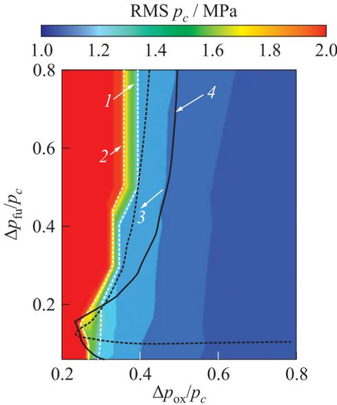
**Figure 6** Stability map. Chamber pressure RMS dependency on oxidizer and fuel injector pressure drops: 1 — 10% RMS; 2 — 50% RMS; 3 — analog Szuch; and 4 — experimental
