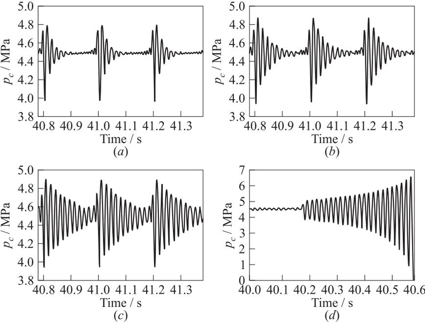
**Figure 4** Double time lag,  $\Delta p_{fu}/p_c = 0.5$ ; time evolution of the chamber pressure response at different oxidizer injector pressure drops: (a)  $\Delta p_{ox}/p_c = 0.5$ ; (b) 0.4; (c) 0.35; and (d)  $\Delta p_{ox}/p_c = 0.3$ , undamped case
