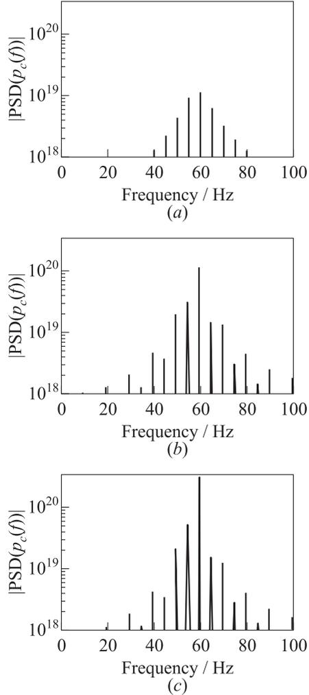
**Figure 5** Double time lag,  $\Delta p_{\text{fu}}/p_c = 0.5$ ; PSD at different oxidizer injector pressure drops: (a)  $\Delta p_{\text{ox}}/p_c = 0.5$ ; (b) 0.4; and (c)  $\Delta p_{\text{ox}}/p_c = 0.35$
