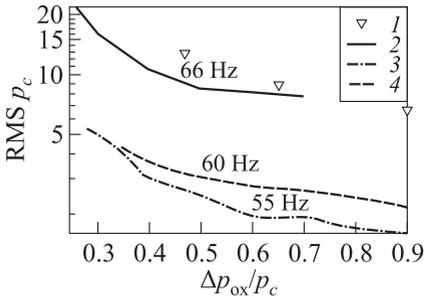
**Figure 2** Double vs. single time lag,  $\Delta p_{fu}/p_c = 0.5$ ; percentage chamber pressure RMS vs. oxidizer injector pressure drops: 1 — experimental; 2 — analog Szuch; 3 — single time lag; and 4 — double time lag
