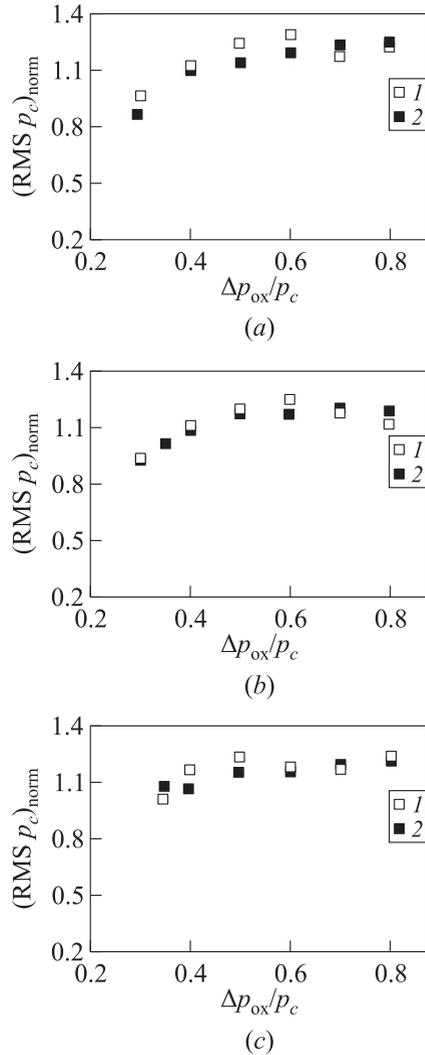
**Figure 7** Double time lag; normalized RMS of the chamber pressure signal for different input amplitudes (1 — +20% and 2 — +100%) at various fuel injector pressure drops: (a)  $\Delta p_{\text{fu}}/p_c = 0.1$ ; (b) 0.15; and (c)  $\Delta p_{\text{fu}}/p_c = 0.4$
