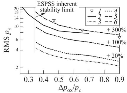
**Figure 3** Double time lag,  $\Delta p_{fu}/p_c = 0.5$ : percentage chamber pressure RMS vs. oxidizer injector pressure drops at different input amplitudes: 1 — experimental; 2 — analog Szuch; 3 —  $\epsilon = 0.01$ ; 4 —  $\epsilon = 0.012$ ; 5 —  $\epsilon = 0.02$ ; and 6 —  $\epsilon = 0.04$
